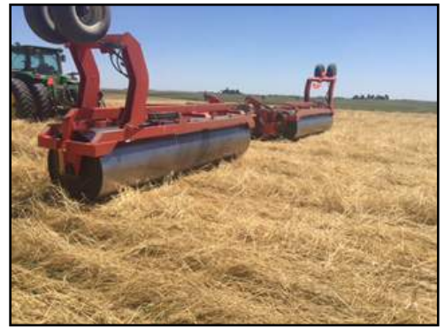
Jack Boyer rolling the chemically terminated cover crop with a RiteWay roller on June 6. Soybeans were seeded on May 16.
