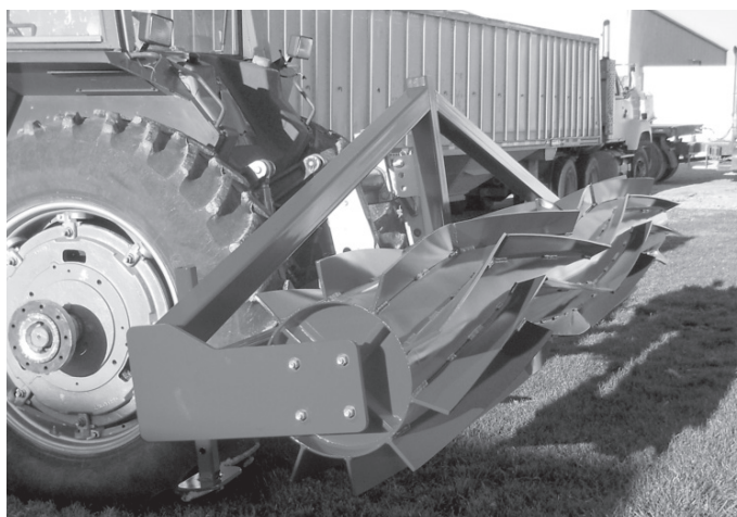
← The roller-crimper Billy and George Naylor had built adopted a double-chevron blade configuration.
