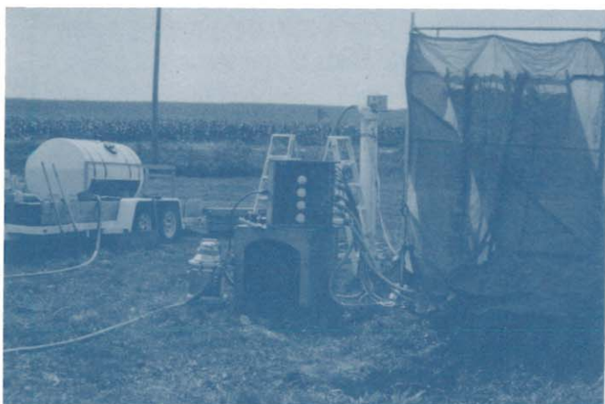
This equipment is used by Tilth Lab researchers to simulate rainfall in the field.
