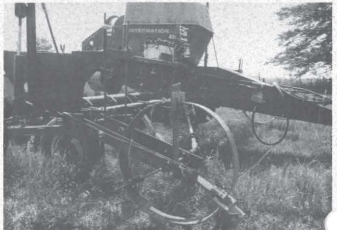
Electronically activated relays drop several seeds per hill. On this prototype, a paddle wheel drives the circuitry and synchronizes the planter with the previous pass.
