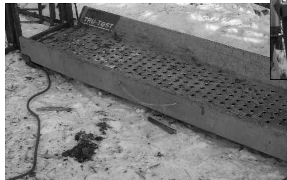
The silver scale shown here connects to an electronic head that displays the weight and stores these values.
