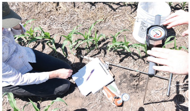
Researchers used a penetrometer to measure soil compaction in Kimberley's corn field on June 6, 2018.
