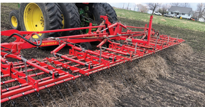
At left, Alert first attempted to use a tine weeder through emerged oats on Apr. 26, 2020 but it resulted in too much plugging. At right, rotary-hoe pass on Apr. 26 that better accommodated the leftover soybean residue from 2019.
