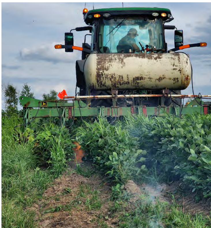
DANIEL FLAME-WEEDING SOYBEANS USING A SIX-ROW FLAME CULTIVATOR KIT MOUNTED TO A CULTIVATOR TOOL BAR ON JULY 26, 2022. DANIEL'S ORIGINAL PLAN WAS TO FLAME-WEED EARLIER IN THE SEASON.
