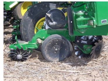
Planter Settings for Sowing Corn and Soybeans Into Covers
