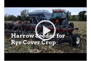
Will Cannon of Prairie City, Iowa, has improvised a method for seeding cover crops quickly and inexpensively. The setup: a Hiniker air seeder with Gandy seed meters mounted on a frame he made that pulls a preowned J&M double-rolling harrow.
