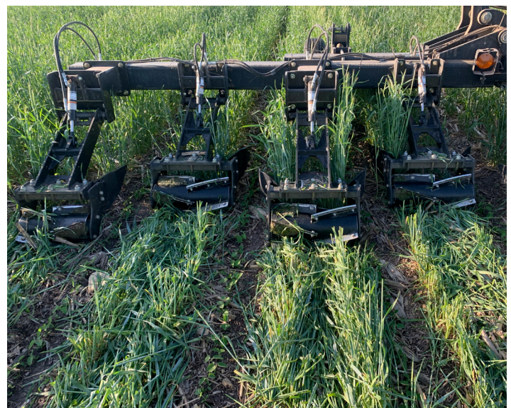
Michael Vittetoe's in-row roll-crimper in action crimping rye with undisturbed soybean rows in between the rollers. Photo taken May 16, 2023.
