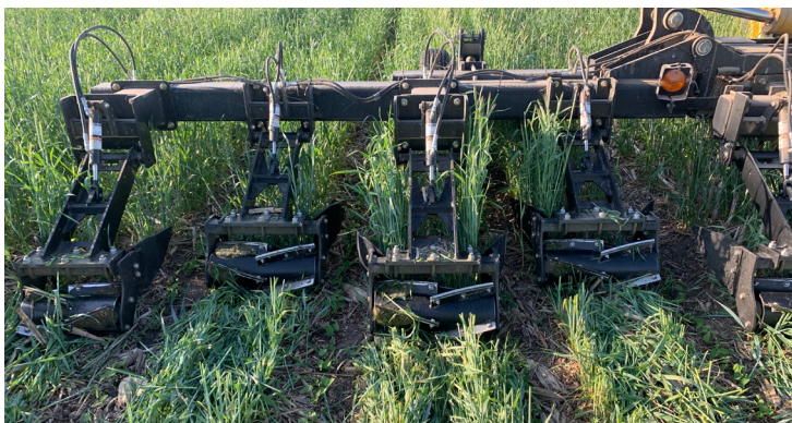
MICHAEL VITTETOE'S IN-RW ROLL-CRIMPER IN ACTION CRIMPING RYE WITH UNDISTURBED SOYBEAN ROWS IN BETWEEN THE ROLLERS. MICHAEL SEEDED A COVER CROP IN 10-INCH TWIN-ROWS ON 30-INCH CENTERS SO HE CAN PLANT SOYBEANS BETWEEN COVER CROP ROWS. PHOTO TAKEN MAY 16, 2023.
