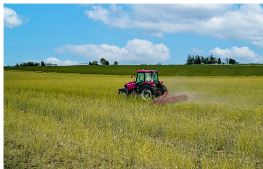
FRED ABELS USING HIS ROLLER-CRIMPER TO TERMINATE CEREAL RYE AT GRAIN FILL. PHOTO TAKEN JUNE 14, 2023 BY BRADY APPEL.
