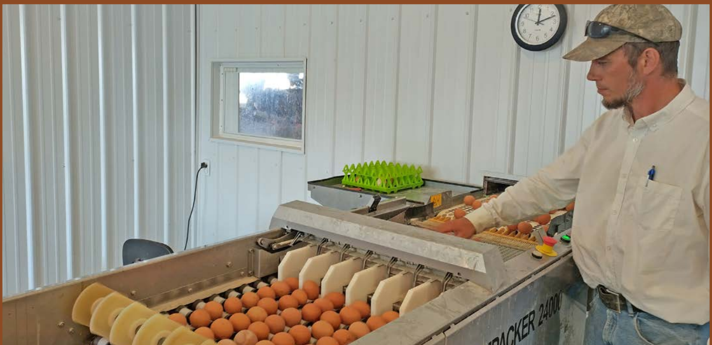
The nest boxes are angled so that the eggs roll onto the conveyor belt where Arlyn watches for any defects.
