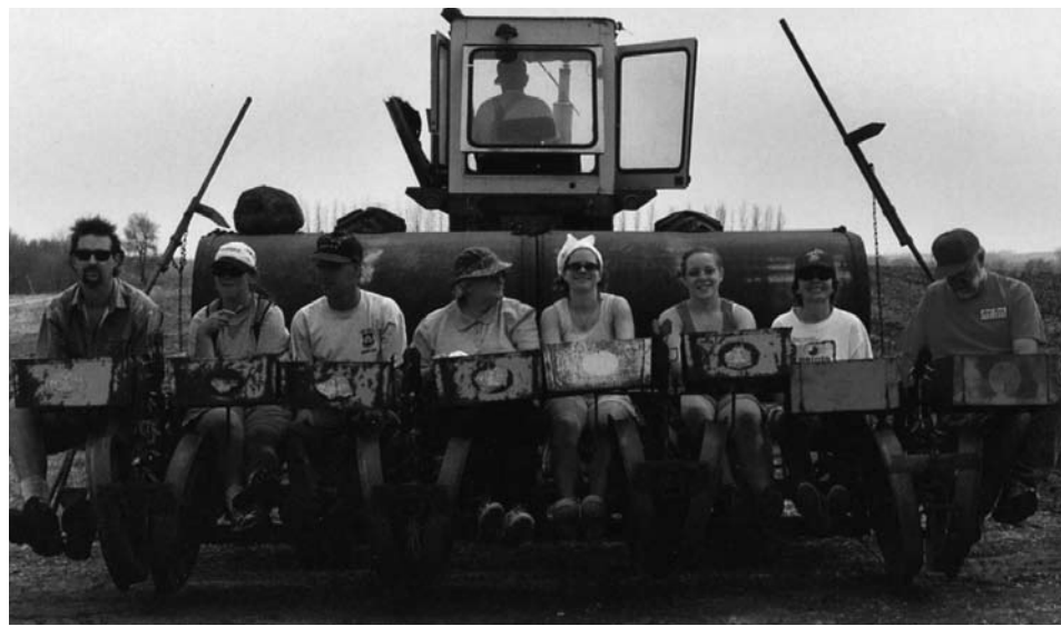
Machinery makes it possible for the Berry Patch to produce more than 40 acres of fruit. With the four row transplanter above, eight people can plant 5,000 plants per hour.
