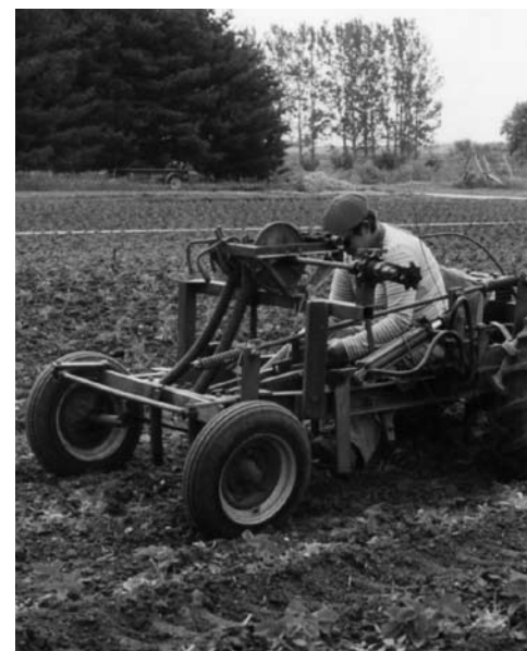
The Friday hoe, above, allows operators to steer with their feet while hand weeding strawberries.
