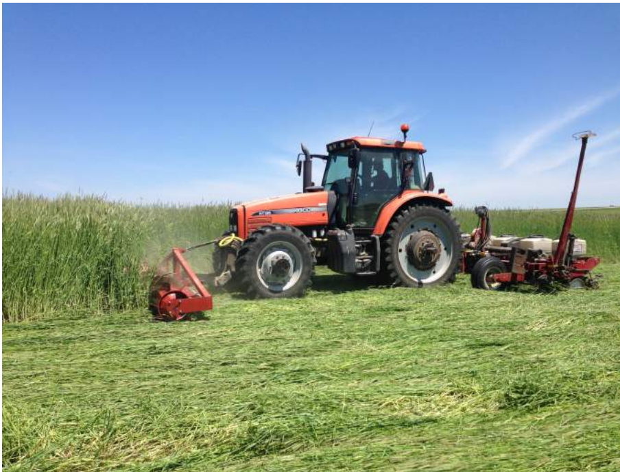
Figure 4. Front-mounted roller-crimper used to terminate cover crops and to create mulches.
