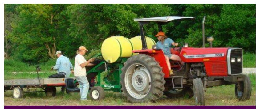
Loading the waterwheel planter, which allows two people to set up to 1000 plants in an hour.
